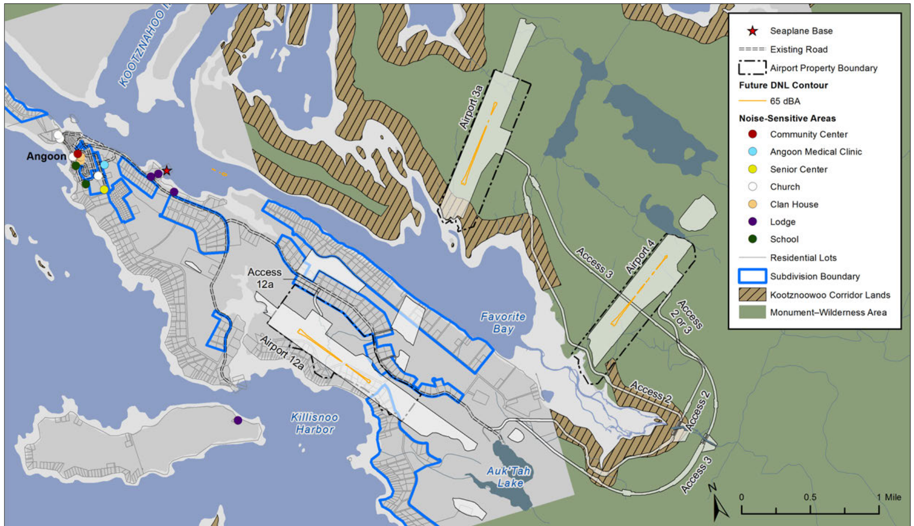
Figure NO7. The noise contour for each land-based airport alternative indicates that noise louder than DNL 65 dBA would not extend beyond the airport boundary.
