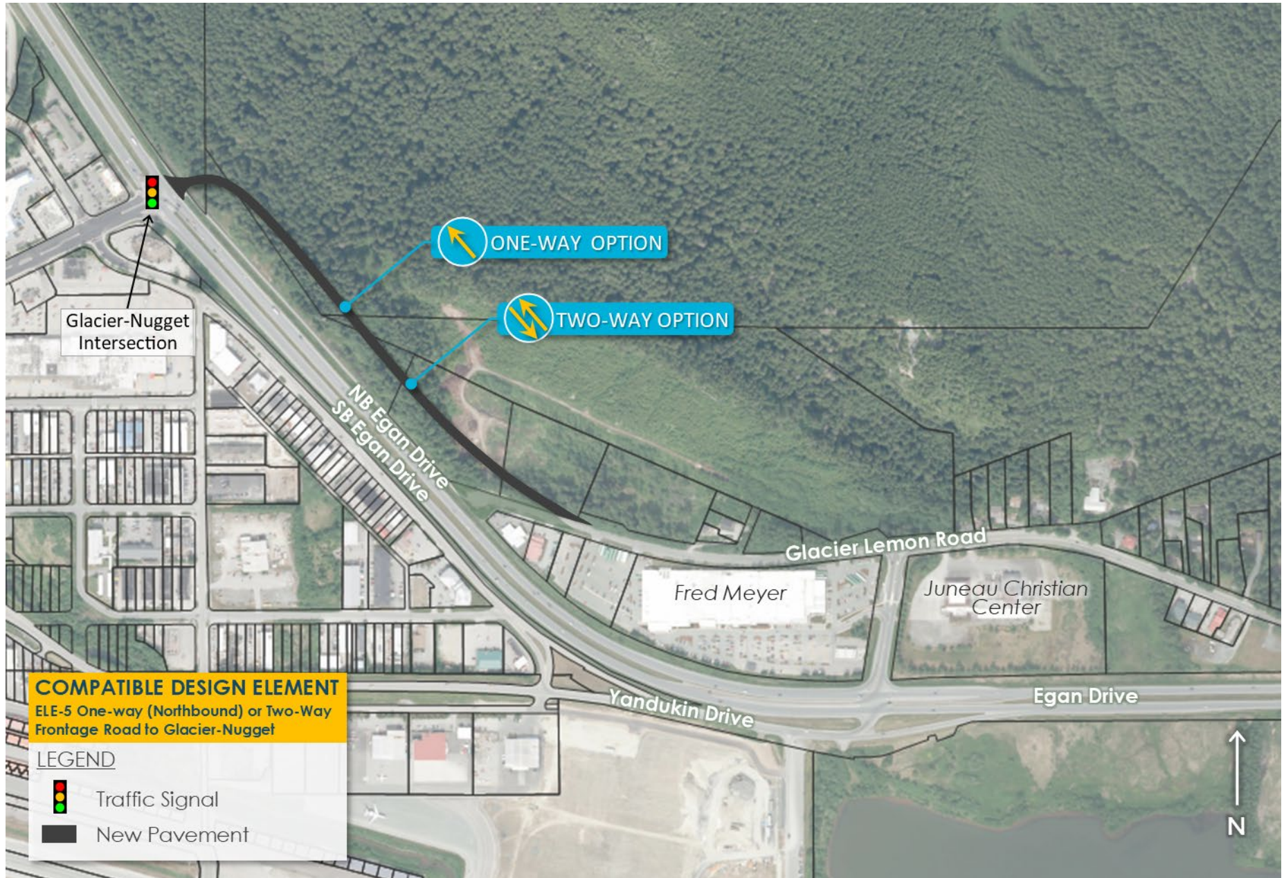
Figure E-2: ELE-5 One-way (Northbound) or Two-way Frontage Road to Glacier-Nugget Diagram
