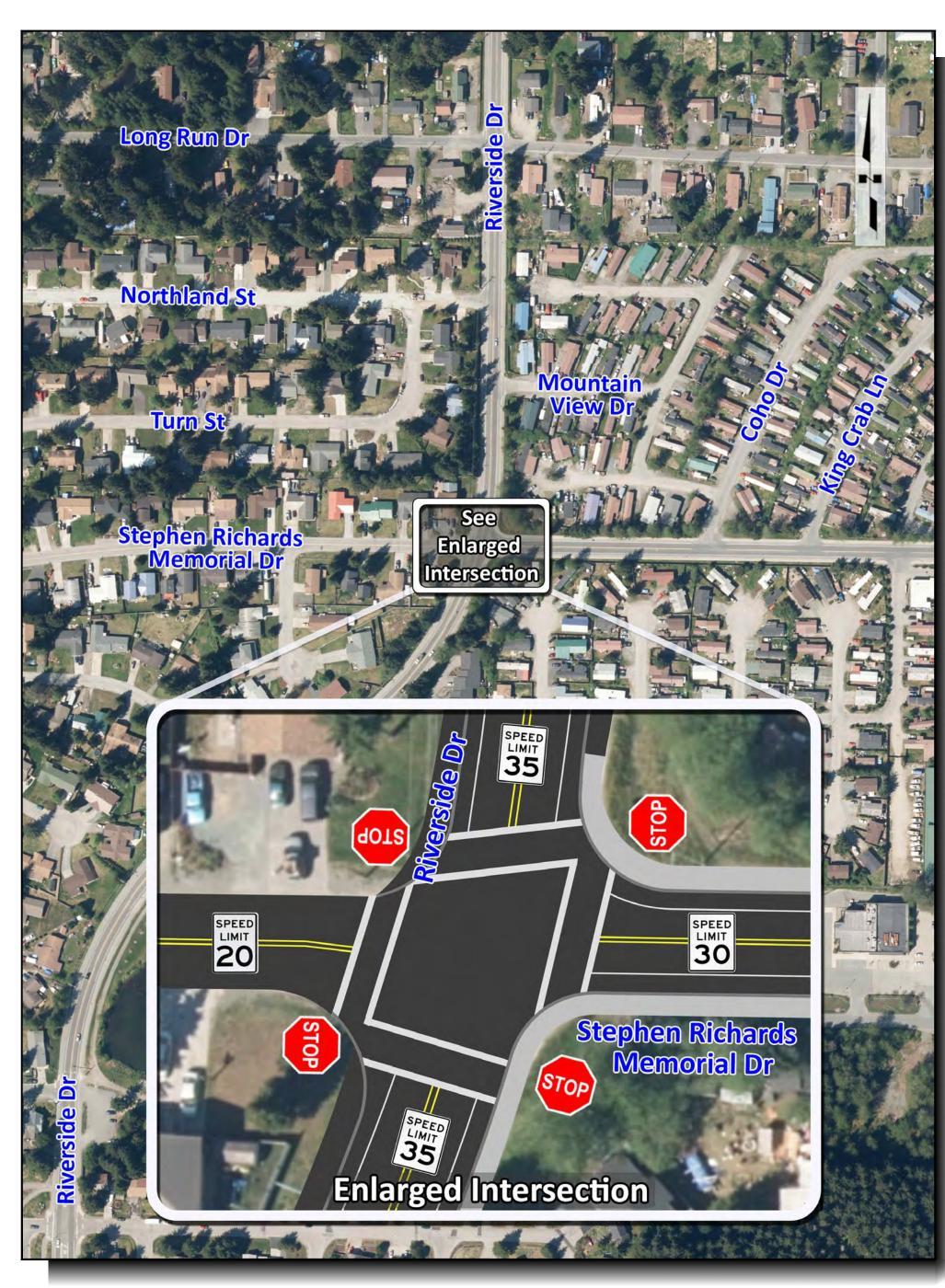
All-way stop with flashing beacon installed in 2008 - crash rate decreased Peak Hour Delay
